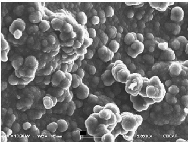
Fig. 11. Micrograph of the as-deposited PANI coating.
